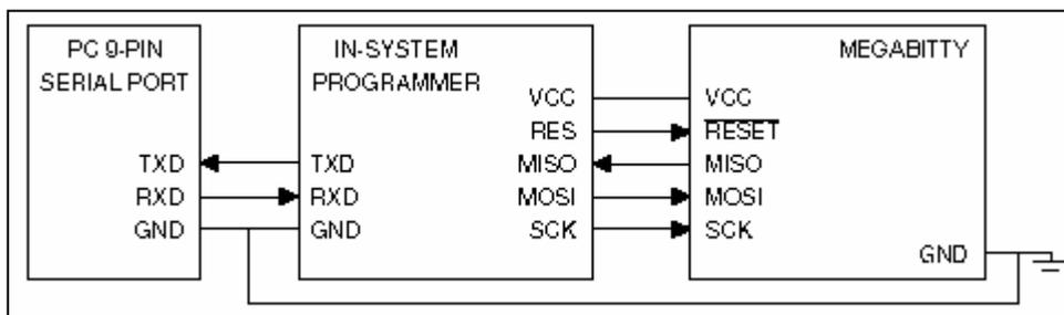
**Figure 1:** The programmer connects to a computer via a serial port, and to MEGAbitty via the ISP connector.
