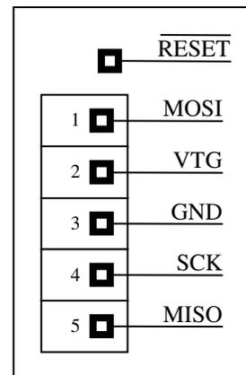
**Figure 4:** MEGAbitty ISP connector. 1x5 0.05” connector; reset line separate.
