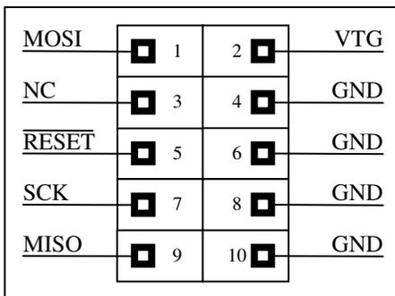
**Figure 3:** Standard 10-pin ISP header. 2x5, 0.10” square-pin connector.
