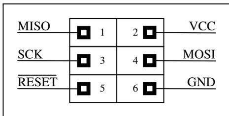
**Figure 2:** Standard 6-pin ISP header. 2x3, 0.10” square-pin connector.
