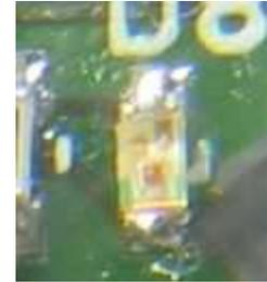
**Figure 4:** Proper LED orientation
