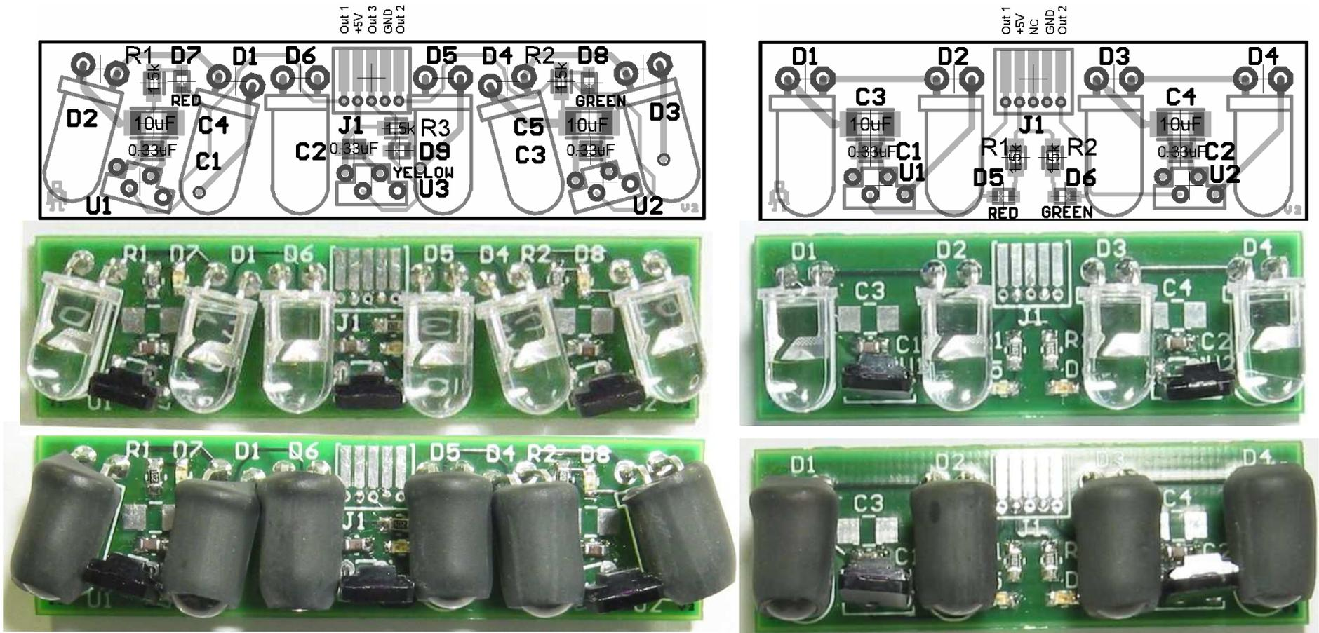
Note that the 10uF caps are not required for proper operation, and are not included in the kit.
