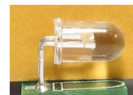
**Figure 5:** Bend LED legs close to base
