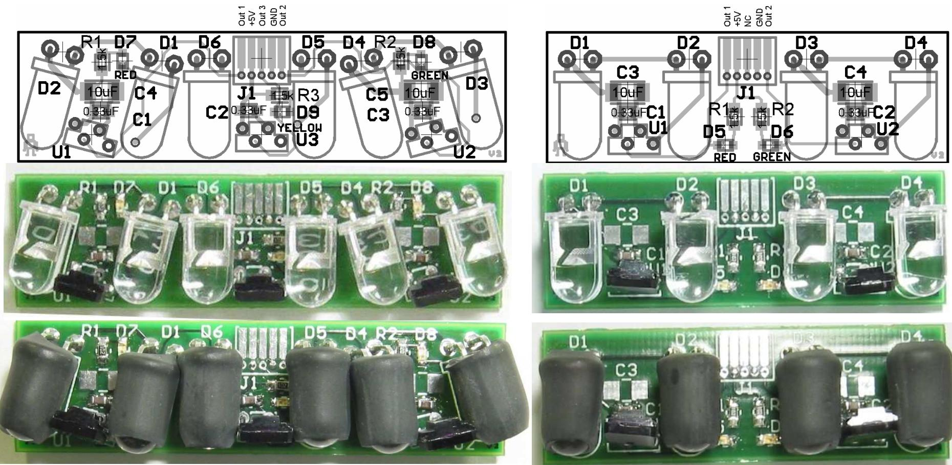
Note that the 10uF caps are not required for proper operation, and are not included in the kit.
